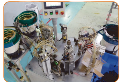
Automated connector production equipment
